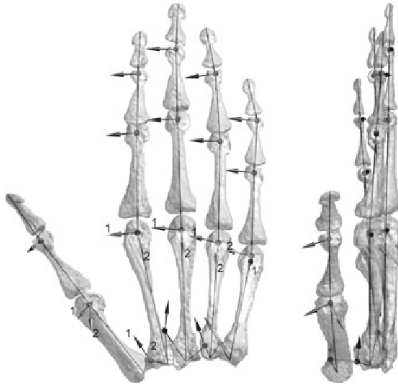
Figure 1: Kinematic model of human hand [9]
