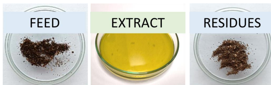
Fig.1. Feed, extract and residues of olive pomace used for supercritical fluid extraction.
