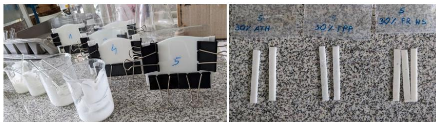
Fig.1. Visual appearance of plasticizer molds and plasticizer shapes with 30 wt.% of flame retardant.
