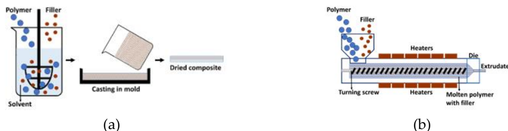
Figure 2.10. Schemes of (a) the solvent casting method and of melt mixing method (b).
