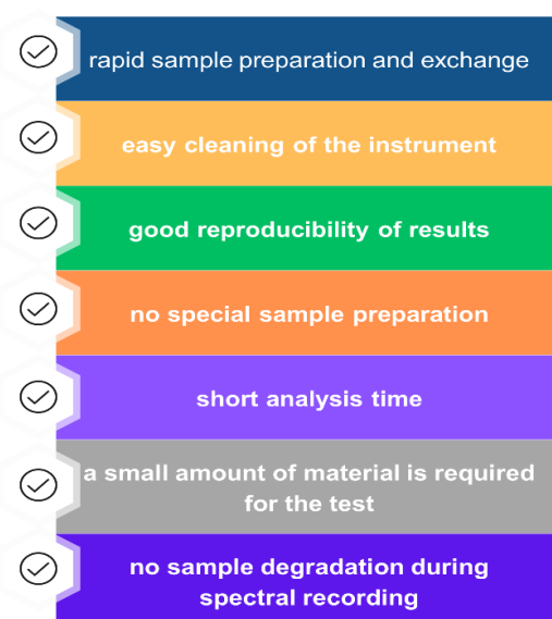
Figure 3.2. Advantages of ATR/FTIR spectroscopy.
